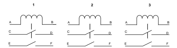
Fig 1. Typical Relay Wiring Diagram (Arrangement looking on front of relay)
